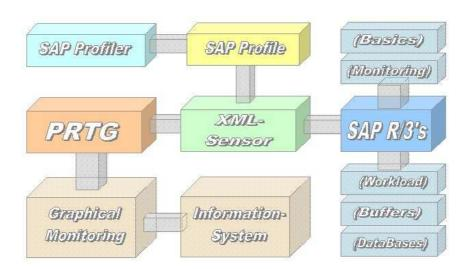
First, the sensor reads out the profile and opens a connection to SAP via RFC (Remote Function Call). With the knowledge of username, password and client it takes a login to SAP. Then the required function is processed within SAP and the resulting is transferred back to the sensor. The sensor formats it and divides it to an information-line and channels. This data are transferred then to the monitoring system.
