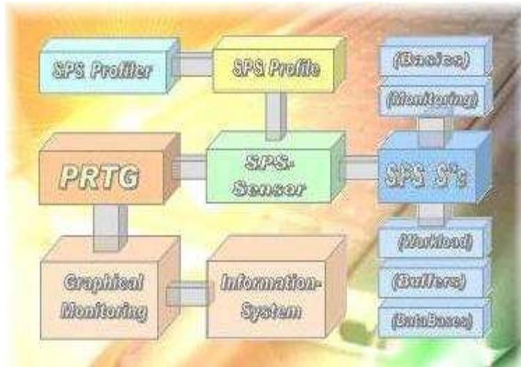
First, the sensor reads out the profile and opens a connection to SPS via RFC1006. With the knowledge of IP-Adress, the Rack- and the Slot-Number the SPS could be accessed. Then the required function is processed within SPS and the resulting is transferred back to the sensor. The sensor formats it and divides it to an information-line and channels. This data are transferred then to PRTG.
